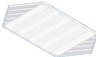
Figure 4: Detail of the plate from heat recovery core
