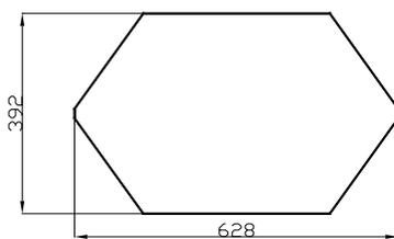
Figure 3: Size of the one plate from heat recovery core
