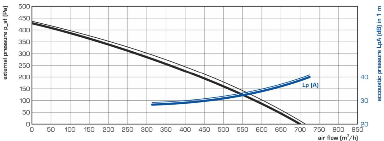
Figure 10: Graph for air performance and sound pressure
