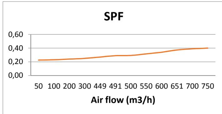
Figure 5: Power consumption for whole unit – two fans and regulation
