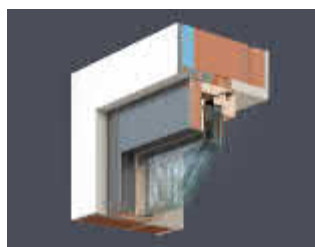
Figure 10: Window installation in existing wall, with insulated jamb panel, window installation partially in front of the façade, exemplary solution of the participant Aluplast.
