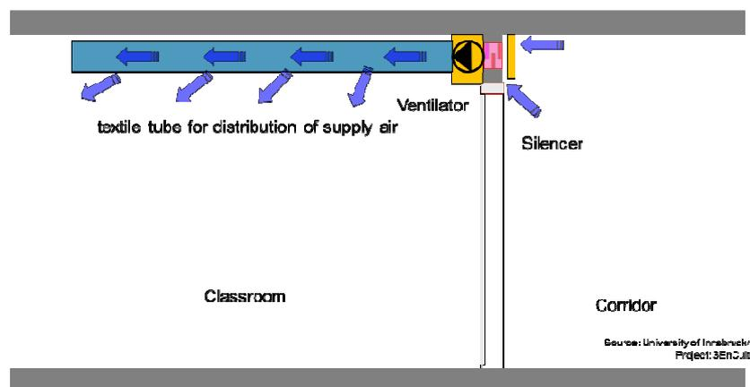
**Figure 1: Principle of active air transfer for non-residential buildings from corridor to class**
