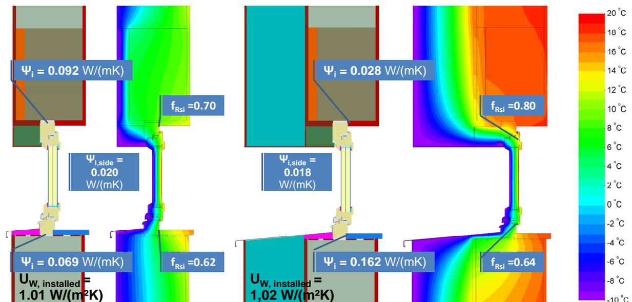
**Figure 2:** Left: With reveal insulation: Significant improvement of both, thermal bridges and temperature factors. Temperature factor at the sill section is still only suitable for warm climate. Right: With reveal insulation and exterior insulation: No changes regarding the U-value of the installed window. Slightly improved temperature factor at the sill profile. Now nearly suitable for the warm, temperate climate.
