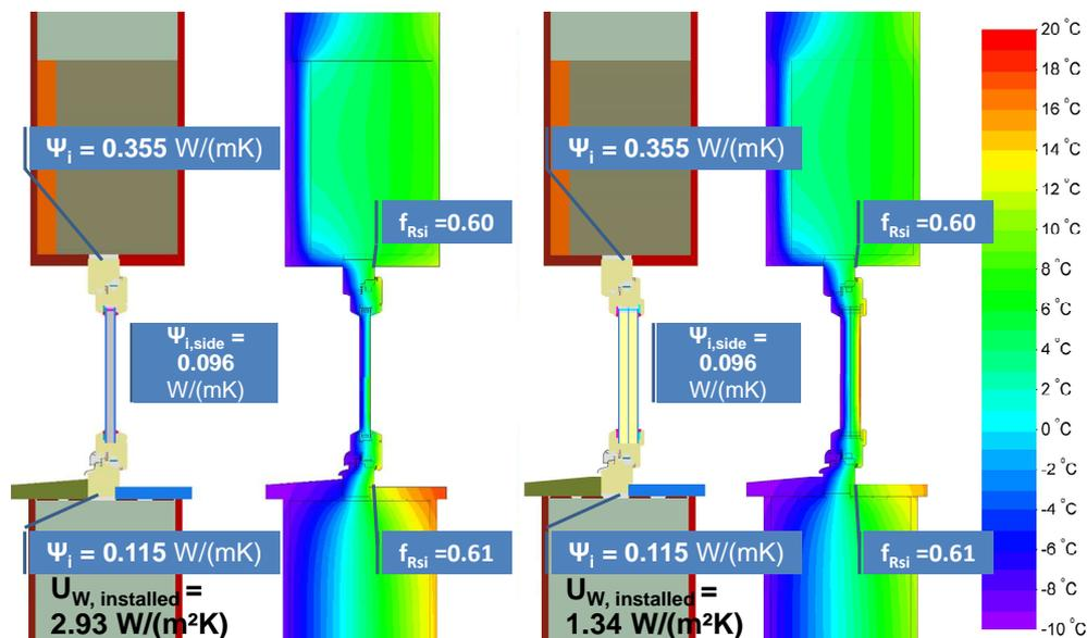
**Figure 1:** Left: Initial situation: Old window in not refurbished facade. Bottom, side and top section of the window: Very high window U-values and thermal bridges are causing unacceptable high thermal losses as well as low temperature factors creating high risk of mould and condensation. Right: The replacement of the glazing is reducing the thermal losses, but not the low temperature factors.
