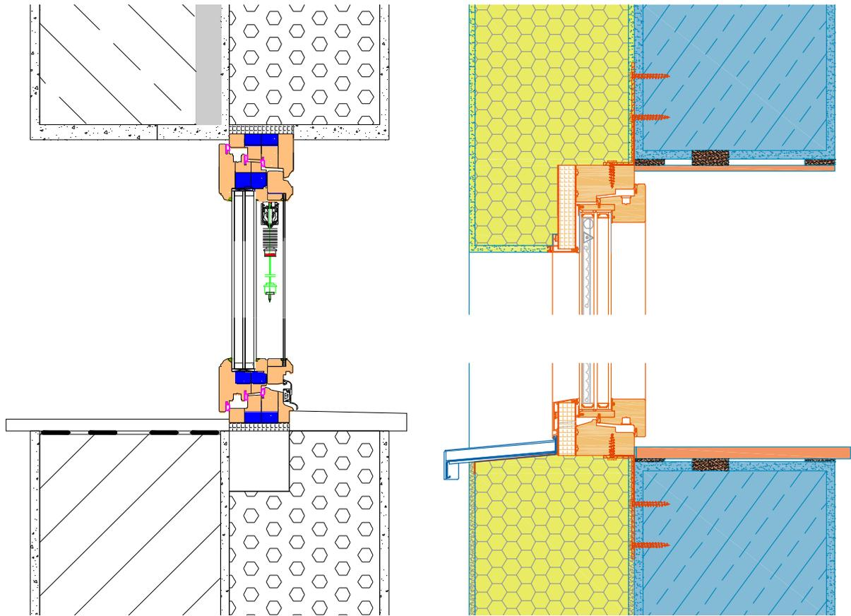
**Figure 4:** Left: Rukna 1 by Bitri: Coupled window with air gap integrated shading. Right: ENERsign plus by Pazen Fenster und Technik: With gas gap integrated roller blind.
