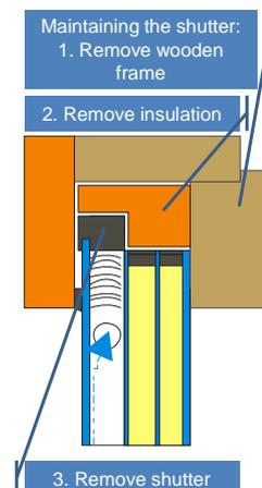
**Figure 2:** Principle solution for fixed frames
