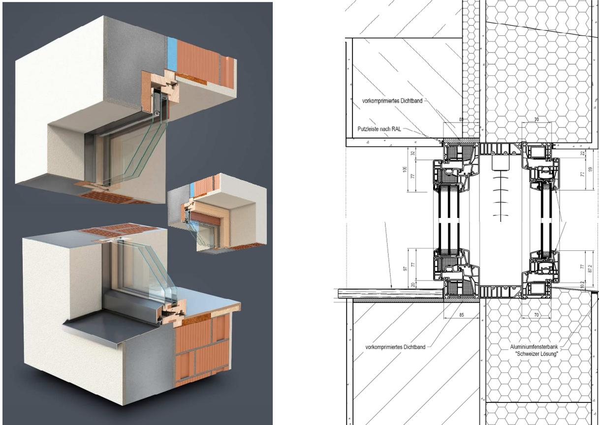
**Figure 3:** Left: Smartwin compact S by pro Passivhausfenster: Solution with air gap integrated shading as proposed in this document. Right: Aluplast: Casement window.
