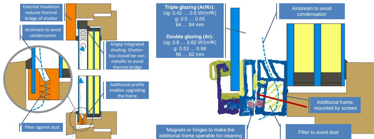
**Figure 1:** Left: Airgap integrated shading in principle. Right: Schematic solution for an additional frame.
