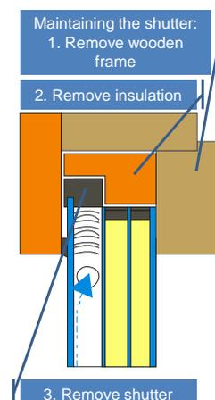
**Figure 2:** Principle solution for fixed frames
