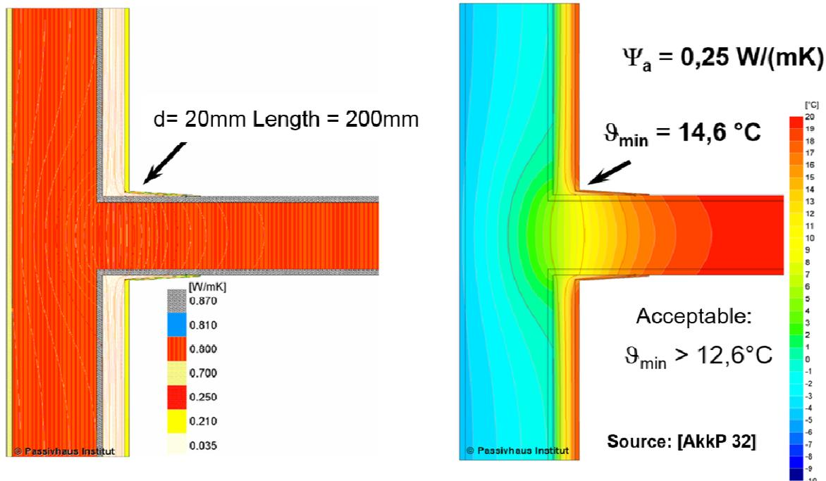
In this case, a “wedge” in the intersection between the wall and the slab allows for a higher surface temperature, reducing the risk of mold formation and/or structural damage.
