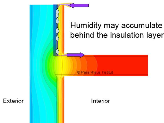
**Figure 1 Faulty execution of interior insulation may lead to moisture problems and increased risk of structural damage.**
